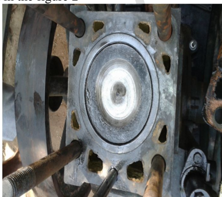
Figure 2 photographic view of employed toroidal combustion chamber
